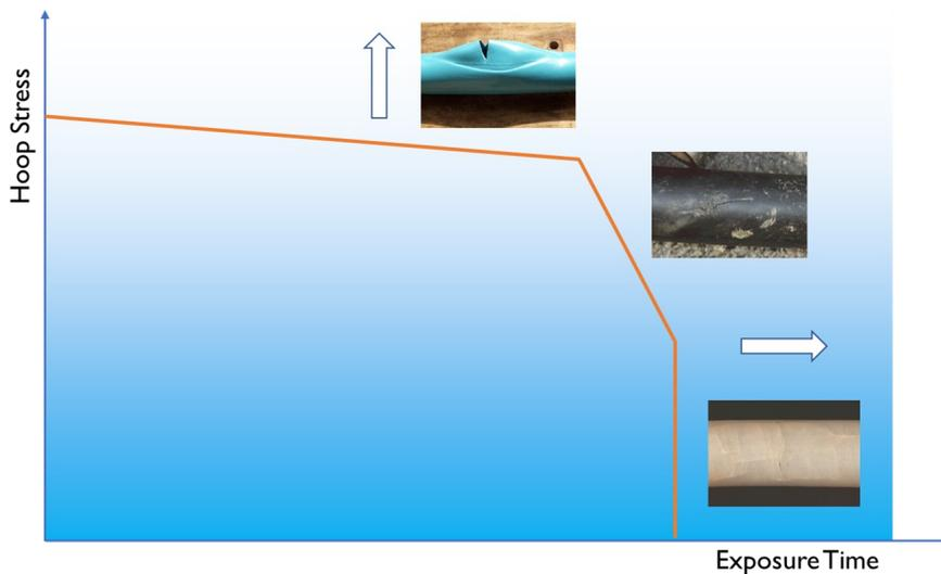
An envelope of performance can be constructed, using Arrhenius' equations, describing when these failure modes can occur in time.
