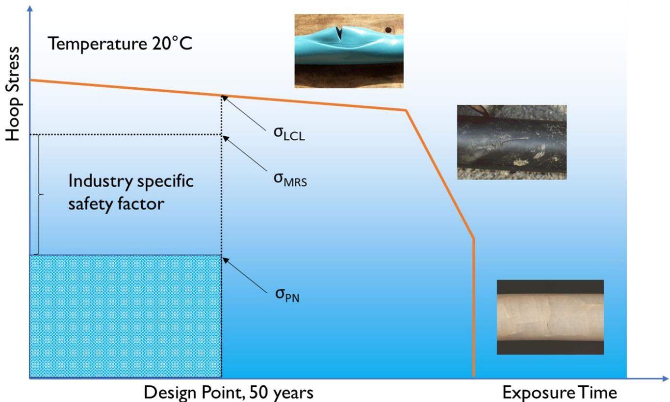
So, the 50-year classification systems means the pipe is operating a long way from the predicted failure points.
