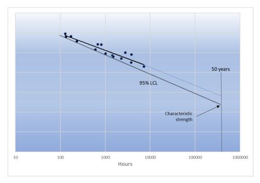
A designer can compare the characteristic strengths with the expected loads (with many safety factors included) to ensure that the installation does not fail either by collapse or by deflecting more than allowed at the surface.
