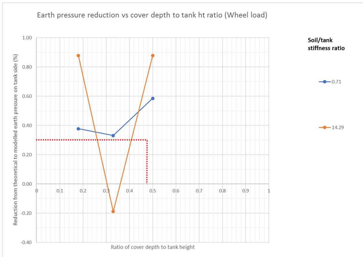
Figure E.4 Earth pressure reduction vs depth:tank height for wheel loads
