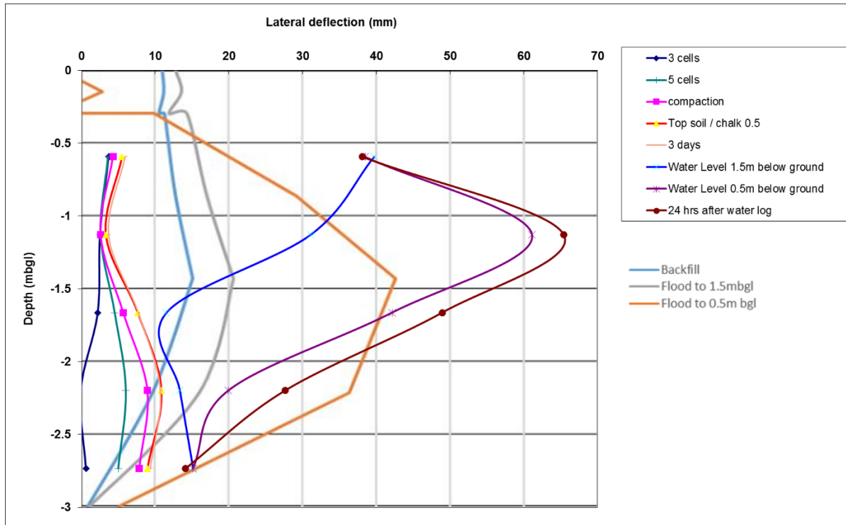
Figure E.2 Comparison of predicted with actual movements
