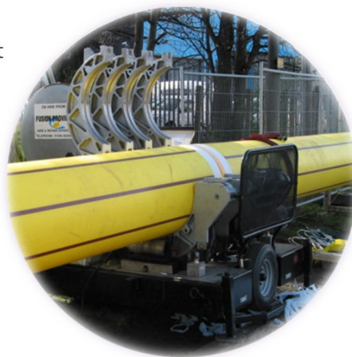
A fully automatic butt fusion welding machine for 630mm diameter polyethylene pipe systems
